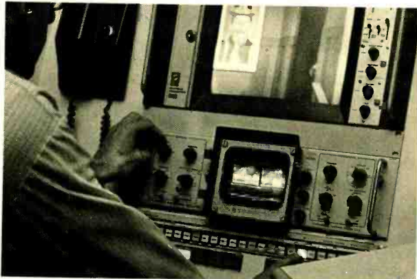
Signal quality evaluation position manned by Chief Engineer, Gary Horrocks. Any source, including individual cameras, KTVX transmitter, and competition can be selected for display.
